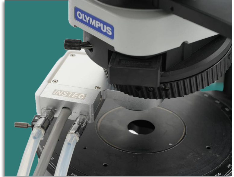
Figure 1. TP102-OBJ mounted on an objective.
