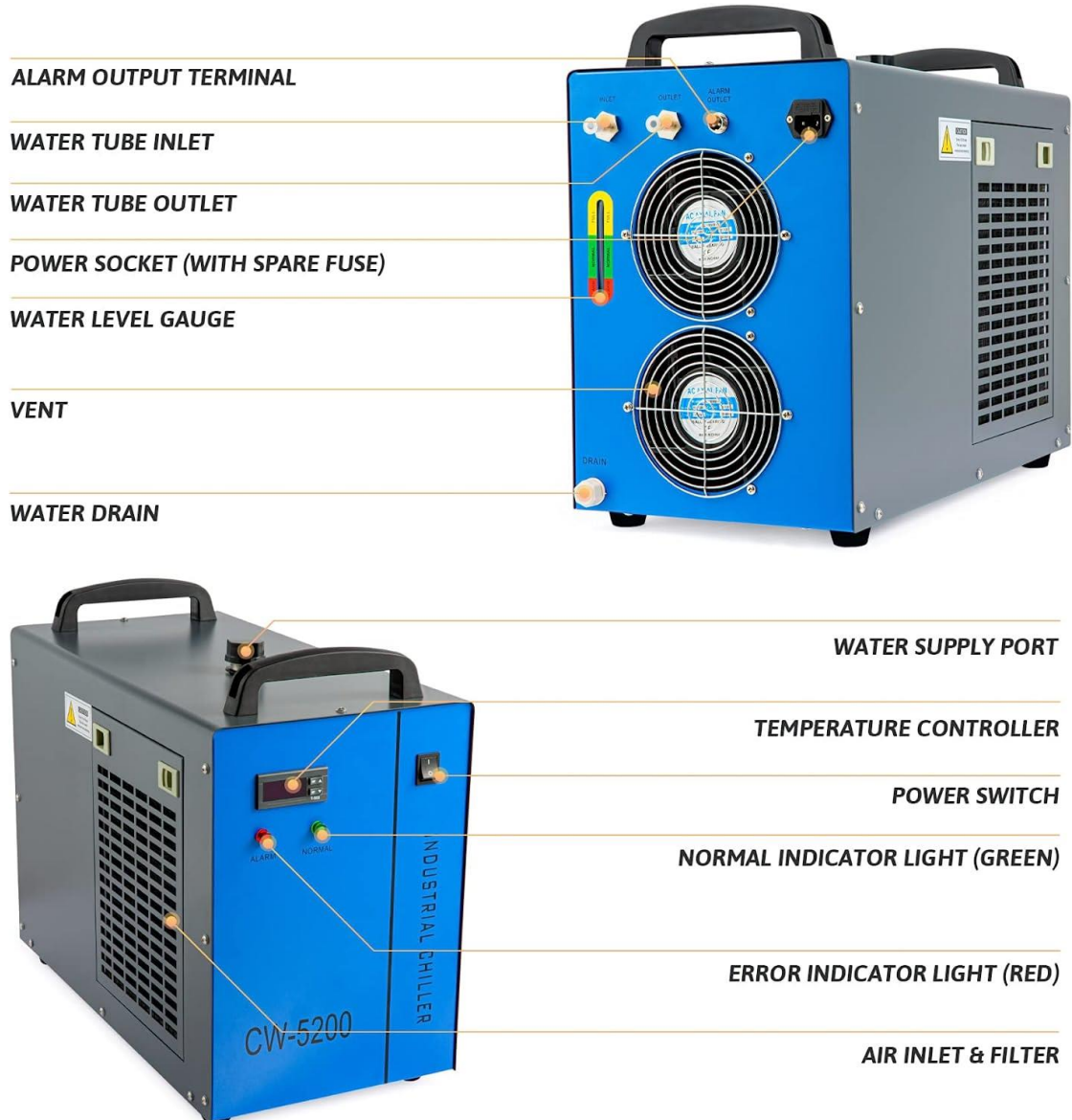
Figure 4: CW5000 Overview Diagram
