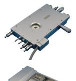
**HCS601GXY-IRM** FTIR heating and cooling stage with 24mm x 24mm sample area. Temperature Range -190°C to 600°C. Gas tight chamber with gas purge capabilities. CWD=10.5mm WD=10.5mm, cone angle>100°C. Includes IR windows. Has a wider temperature range, sealed chamber, and integrated XY sample positioning. Optimized for IR applications.
