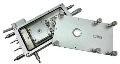
making it possible to re-position samples while maintaining a controlled atmosphere. The standard XY sample holder is designed for use with 25mm x 75mm glass slides, but custom XY tongues for other samples are available upon request. Vertical mounting orientation is also available with customization.
