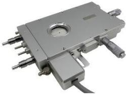
**HCS621GXY** heating and cooling stage with 28mm x 28mm sample area. Temperature range from -190°C to 600°C. Gas-tight chamber with gas purge capabilities. Includes XY positioning and option to add electrical feedthroughs. Offer greatly increased temperature range over TS102S but requires LN2 cooling, larger working distance, and is optimized for upright microscopy.
