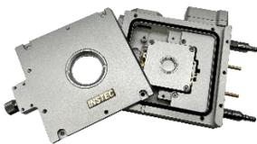
**TP102G** Gas-tight heating and cooling plate. -30°C to 120°C without consumable coolant such as LN2. Optional inner lid for maximizing temperature uniformity. Offers gas-tight sample area to prevent condensation, but requires smaller sample sizes than the TS102S and does not have a transmission aperture. For transmission capability, see **TS102VXY**.
