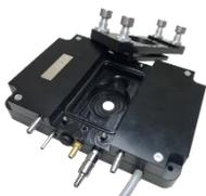
**TSA12Gi** Thermoelectric heating and cooling plate for inverted optical microscopy. Gas-tight chamber supports 25mm by 75mm glass slides, or 35mm petri dishes. Temperature range -25°C to 120°C. 5.4mm minimum objective working distance, 22.8mm minimum condenser working distance. 12mm diameter transmission aperture. Offers improved performance over TS102S, and supports petri dishes, but requires longer working distances. Optimized for inverted microscopy.
