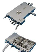
**HCS601GXY-IRM** FTIR heating and cooling stage with 24mm x 24mm sample area. Temperature Range -190°C to 600°C. Gas tight chamber with gas purge capabilities. CWD=10.5mm WD=10.5mm, cone angle>100°C. Includes IR windows. Has a slightly smaller sample area, and is optimized for IR applications.
