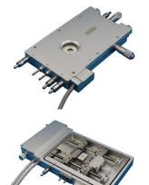
HCS601GXY-IRM FTIR heating and cooling stage with 24mm x 24mm sample area. Temperature Range -190°C to 600°C. Gas tight chamber with gas purge capabilities. CWD=10.5mm WD=10.5mm, cone angle>100°C. Includes IR windows. Has a wider temperature range, but a slightly smaller sample area, and is optimized for IR applications.
