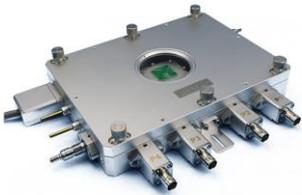
**TP102V-PM** thermoelectric mini probe stage with 40mm x 40mm sample area. Temperature Range -25°C to 150°C. Low-vacuum tight chamber with gas purge capabilities. Probes not movable with cover lid on. Option to add electrical feedthroughs..
