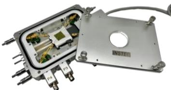
**HCP621G-PMH** hall effect measurement stage with 28mm x 28mm sample area. Temperature range -190°C to 400°C. Low-vacuum tight chamber with gas purge capabilities. Probes not movable with cover lid on. Option to add electrical feedthroughs.
