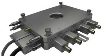
**HP1000V-PM** high-temperature mini probe stage with 16mm x 16mm sample area. Temperature range ambient to 1000°C (heating only). Low-vacuum tight chamber with gas purge capabilities. Probes not movable with cover lid on. Option to add electrical feedthroughs.
